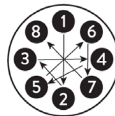
8 Compression Hex Nut Tightening Pattern
