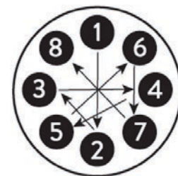
8 Compression Hex Nut Tightening Pattern
