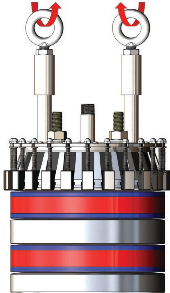
Figure 18: Properly Installed Lifting Eyes for Vertical Lifting
