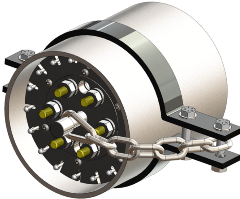
Figure 26: Properly Installed Safety Gag on Pipe
