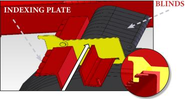
Ensure that the key is properly inserted in the indexing plate slot to prevent movement of blinds
